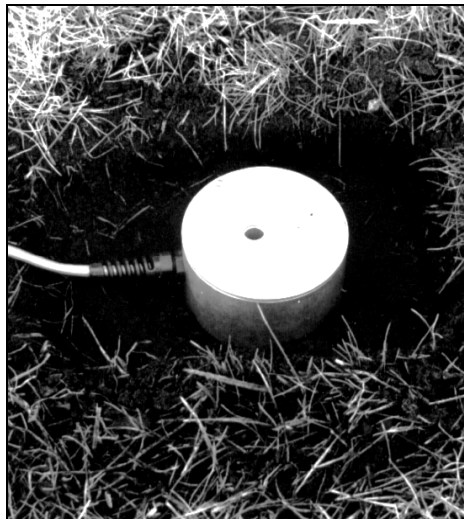
Figure 3.8 Burying the Standard Transducer.
