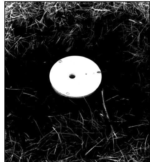
Figure 3.9 Fill In and Pack the Material around the Standard Transducer.
