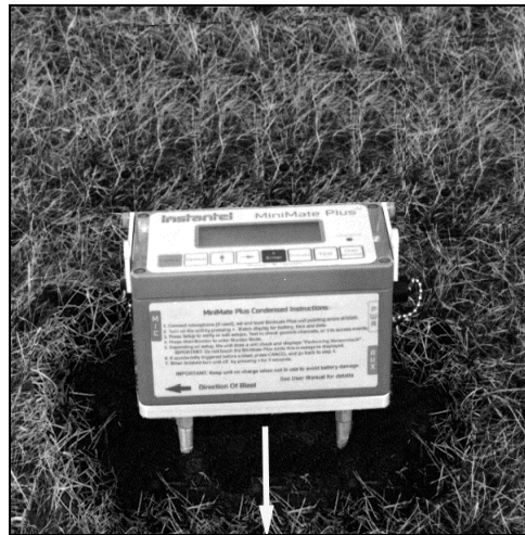
Figure 3.2 Installing the MiniMate Plus using the Ground Spikes.
