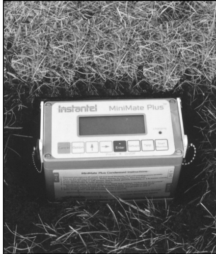
Figure 3.6 Burying the MiniMate Plus. Protect the Monitor with a Plastic Bag.
