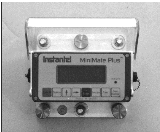
Figure 5.5 Installing the MiniMate Plus on a Ceiling using the Fastening Plate.
